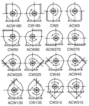
Direction of rotation is determined from the drive side. On single inlet fans, drive side is considered as opposite inlet, regardless of actual drive location.
