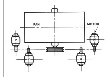
The location of motor is determined from plan view of the blower, designating the motor position by letters W, X, Y and Z as the case may be.
